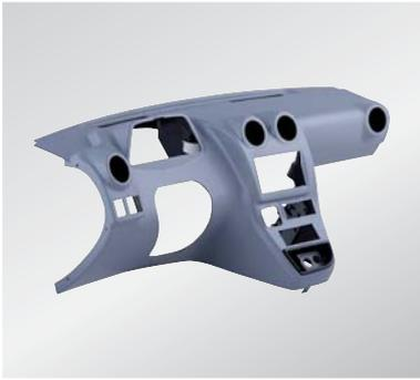
Dashboard for special vehicle with mounted applications and mounts at the rear
